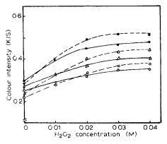
Fig. 1. Relationship between colour intensity of the dyed substrates and the concentration of H<sub>2</sub>O<sub>2</sub> present in the dyeing medium. Dyeing: 2% o.w.f., 75°C, pH 4, 1 h, liq. ratio 100:1; thiourea 0.05 m. ——, CI Acid Blue 23; ——, CI Acid Red 85; ●, wool; △, silk; ○, polyamide-6 fabric.
