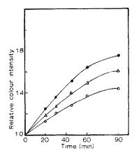
Fig. 2. Relationship between the relative colour intensity of the dyed substrates and the time of dyeing at 75°C in the presence of  $H_2O_2$  (0.03 M)/thiourea (0.05 M) redox system. Dyeing: CI Acid Blue 3, 1% o.w.f., pH 4, liq. ratio 100:1.  $\blacksquare$ , Wool;  $\triangle$ , silk;  $\bigcirc$ , polyamide-6.
