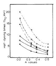
Fig. 4. Relationship between half-dyeing time of dyed substrates and the A value of the acid dyes. Dyeing: 3% o.w.f., 80°C, pH 4, liq. ratio 100:1, H<sub>2</sub>O<sub>2</sub> (0·03 m)/thiourea (0·05 m). ---, Aqueous medium; —, water/propanol (9:1) mixture medium; ●, wool; □, silk; ×, polyamide-6.
