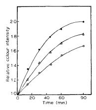
Fig. 3. Relationship between the relative colour intensity of dyed substrates and the time of dyeing at 75°C in water/n-propanol (9:1) medium and in presence of H<sub>2</sub>O<sub>2</sub> (0·03 M)/thiourea (0·05 M) redox system. Dyeing: CI Acid Blue 3, 1% o.w.f., pH 4, liq. ratio 100:1. ●, wool; △, silk; ○, polyamide-6 fabric.
